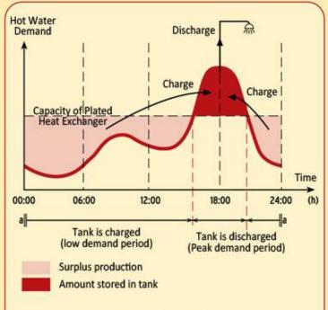
A typical hot water demand profile for an apartment block
