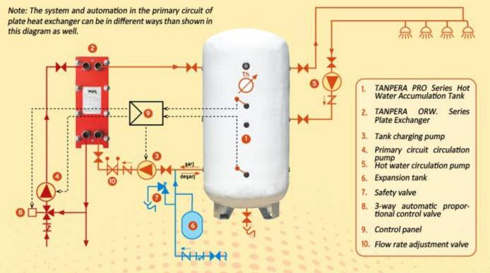
By the installation layout proposed in the above scheme, TANPERA PRO Series Hot Water Accumulation Tank, depending on instant demand, can be discharged regularly by the hot water with desired temperature.
