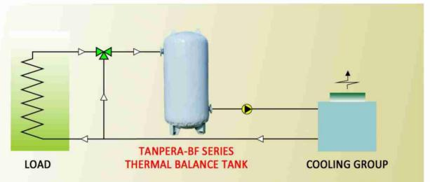
In typical comfort applications where the prevention of over switching of the compressor function of the buffer tank is more important, it is recommended that tank is placed in front of cooling group.
