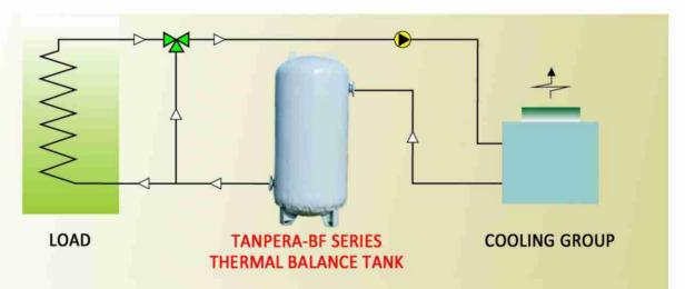
If tank is used in an industrial cooling system, the main purpose is a more sensitive temperature control of the water thus, placing the tank after the group and before the system should be proper.
