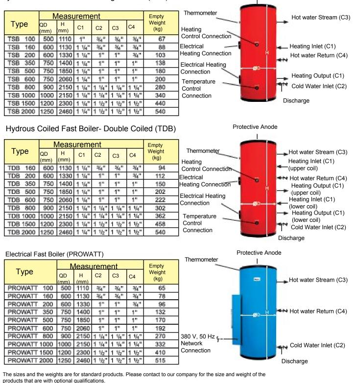
The latest measurement and assembly sizes that can be used in project designing can be viewed in www.tanpera.com.tr
